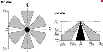
Note: Installation of integrated sensors within 3-ft (1m) of HVAC air vents is not recommended. The pattern shown is intended solely as a general guide and is not to scale.
