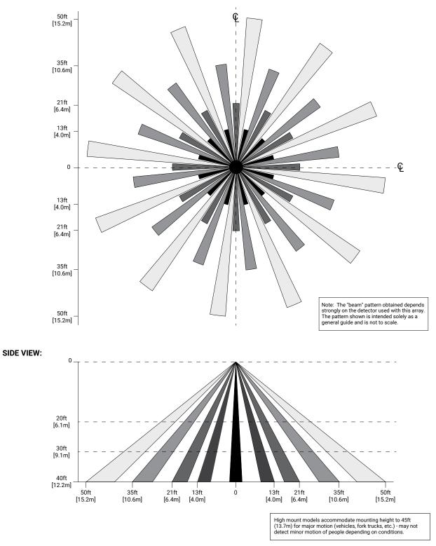
**Note:** False motion detection can occur when objects of contrasting temperature with the surrounding environment move within the sensor field of view. Wind blowing leaves, branches, or other objects can trigger the motion sensor. It is recommended that the sensor be mounted away from these objects.
