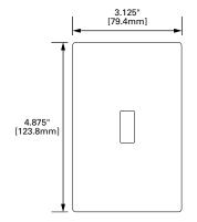
Toggle Wallplates can be used with: Momentary toggle switches, Automatic Turn-Off switches
