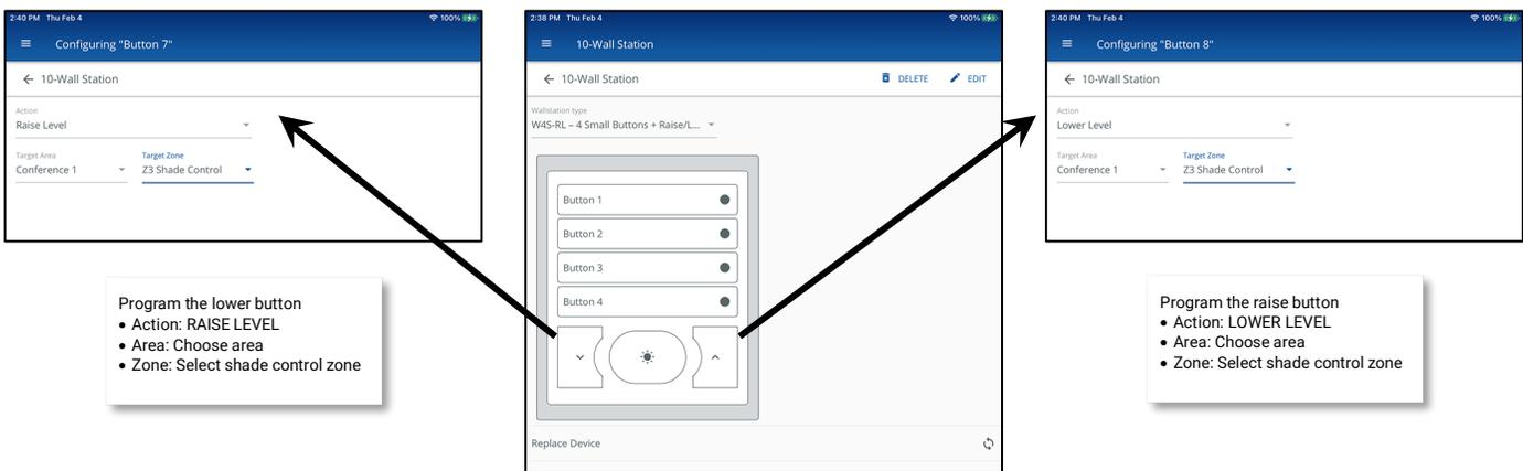
Raise/Lower buttons to adjust shading may not stop the shade when the occupant's finger is removed as the shade may be still in transition between positions. The shade will stop once the position has been executed based on the voltage seen on the 0-10V Input.
