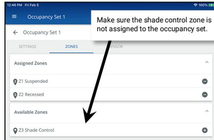
Some sites may want shading to respond to occupancy actions. For instance, the shades could open to the fully open position when the space becomes unoccupied. There may be enough daylight present the next time the space is used to leave lighting off or to reduce the level of electric lighting needed, maximizing energy savings.
