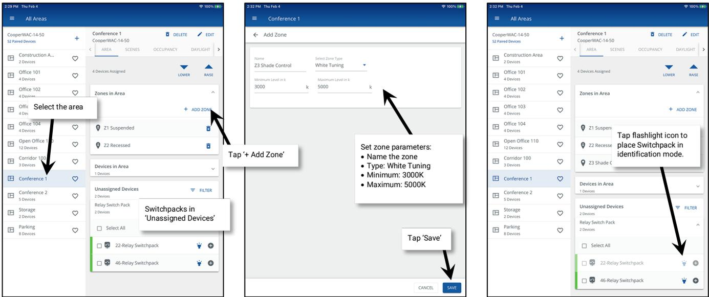
4. Manually select the Switchpack (make sure it is the only device selected) and then tap the '+' icon or '+ Add' option. When prompted, select to add the device **to the AREA** (not the shading zone). Locate the assigned Switchpack in the 'Devices in Area' section, and then tap the device to open it.
