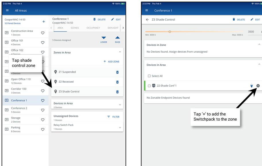
8. Once the device is assigned, test the shade operation by using the zone adjust bar.
