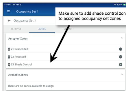
Then, program the shade control zone level into the scene that is being used for the appropriate occupied and/or unoccupied action. If only one of the actions triggers the shade response, make certain to ignore the shade control from the other action's scene.
