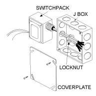
All connections are made via pigtails with twist-on wire
