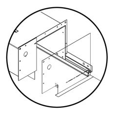
If the wall rail extends more than three inches past the end of the housing, install a support strap as shown.
