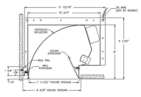
Cut the wall extrusions to fit the total run length. Using screws, mount each to the wall as shown, making sure each is flat and level for best appearance. Cut the fixture's wall rail to fit the total run length, so it is centered in the desired space.
