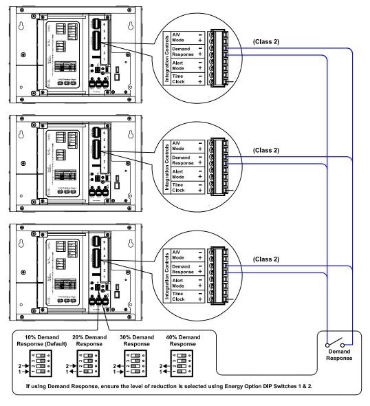
Control Sequence: Demand Response input ensurs light level reduction based on Energy Option DIP switch setting at each Room Controller. The light level reduction occurs regardless of Occupancy, Daylighting or Wallstation current setting. Demand Response light level reduction reduces lighting at a 5% dimming rate to limit occupant impact.
