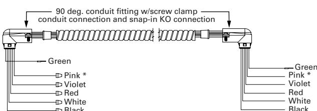
\* Constructions built before Jan 2022 may have gray wire for 0-10 dimming control present. In these cases, the installer will label the gray building wire as a 0-10 dimming wire and connect to our product's pink 0-10V dimming control wire. Reference NFPA70 (2020 NEC), section 410.69.
