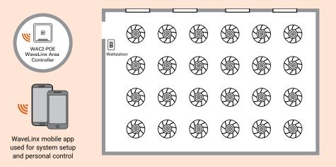
Out of the box operation Occupied to 100%, Unoccupied to 10% Commissioning provides Occupancy / Vacancy Closed loop daylighting Continuous dimming Manual Controls Scheduling (including Astro) UL924 Energy calculations available through WaveLinx CORE DLC BLC V5 qualified
