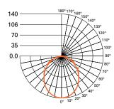
Test Information File Name: CS-SL-9SCT-120-ID-UNV-W-SA-STD-1F-(Low-4000K) Test Method: LM-79-2019 Report Number: P861226 TEST IS SCALED FROM IESNA LM-79-08 TEST DATA (G2-2312-259-1) 1FT Selectable Settings: 4000K CCT, Low Output Luminaire Lumens: 378.7 lumens Efficacy: 108.2 lumens/watt
