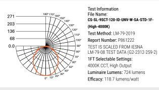
Luminaire Lumens: 724 lumens Efficacy: 118.7 lumens/watt Test Information File Name: CS-SL-9SCT-120-ID-UNV-W-SA-STD-4F-(High-4000K) Test Method: LM-79-2019 Report Number: P861230 TEST IS SCALED FROM IESNA LM-79-08 TEST DATA (G2-2312-259-4) 4FT Selectable Settings: 4000K CCT, High Output Luminaire Lumens: 2740.2 lumens Efficacy: 133 lumens/watt
