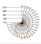
**Test Information** File Name: CS-SL-9SCT-120-ID-UNV-W-SA-STD-4F-(Low-4000K) Test Method: LM-79-2019 Report Number: P861234 TEST IS SCALED FROM IESNA LM-79-08 TEST DATA (G2-2312-259-3) 4FT Selectable Settings: 4000K CCT, Low Output Luminaire Lumens: 1390.5 lumens Efficacy: 132.4 lumens/watt
