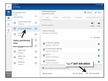
3: Select the sub area to adjust and select the Zones tab. Tap • Add to assign a sub zone to the sub area. Tap • Remove to unassign a sub zone to the sub area.
