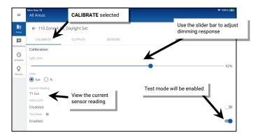
6: Once the adjustment is complete, enable or disable the daylight set to **DIM to OFF** (see "Enabling/Disabling DIM to OFF Capability for Open Loop Daylight Sets" on page 283 for further details). 342,343 Then disable **Test Mode** or allow it to automatically time out after 10 minutes. Tap the back button to exit the calibration screen. Adjusted light level settings are automatically saved.
