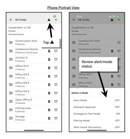
Test Mode will automatically time out after the user defined period expires. To cancel Test Mode before the time expires, either tap **STOP TEST** in the Test Mode screen, or from the Emergency Mode screen, tap the **TESTING NaN:00** button and select **STOP TEST** from the drop down.
