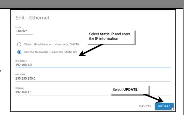
Once the remaining steps of configuration are complete, if IP addresses of the Area Hub(s) have been changed to a different subnet, remember to change the WaveLinx Area Controller's IP address to a static IP on the new subnet.
