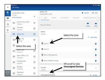
3: In the Unassigned Devices section, identify and then select the desired device(s). Tap • ADD to move the device(s) into the zone or area.
