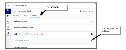
5: Adjust the Associated Occupancy Level to the desired level and then tap SAVE.
