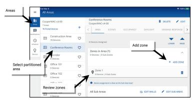
3: Type a descriptive name for the zone, and then select the zone type (dimmable, non-dimmable [switched], receptacle, or white tuning). **Zone type cannot be changed after initial setup**.
