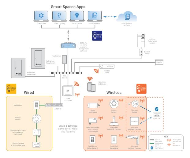
Regardless of what size system is being implemented, or which components are being used, it will be necessary to start by adding the devices to the appropriate WaveLinx Area Controller. Use this user manual to:
