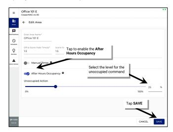
For After Hours Occupancy Mode to operate, there must be an After Hours Occupancy action programmed to enable and disable this mode.
