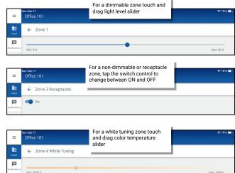
In a partitioned area, this will control levels for all the sub zones that report to that zone regardless of partition wall open or close status. Note: It is not possible to adjust the light level of individual sub zones in a partitioned area. Partition areas may only be accessible to administrator users.
