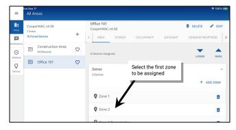
5: In the Zone screen, locate the device in the **Devices in Area** section. Tap • to add the device channel to the zone. The **Multiple Endpoint**Movement screen should display with the chosen zone displayed for the selected channel. Use the drop down for the second channel to select the desired zone for that channel and then tap **SAVE**.
