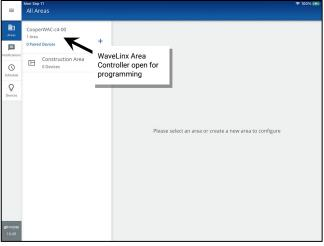
When logging in, if the message displays **WAC CENTRALIZED**, the WaveLinx Area Controller has been added to the WaveLinx CORE System for administration. Before proceeding, make certain to sync the programming from WaveLinx CORE to the WAC before any changes are made. Once changes are complete, make certain that the WAC changes are synced to WaveLinx CORE.
