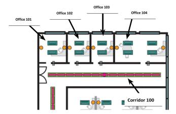
Areas have been created as shown. Each area contains one occupancy set that is defined with a scene command for occupied and unoccupied actions
