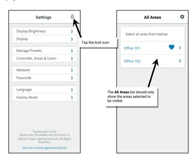
The touchscreen can now be used to control lighting in the defined areas. For information on the screen controls, refer to "Using the Touchscreen Controls" on page 328.
