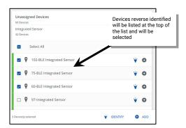
It is also possible to manually select or remove devices from the multi-select by selecting devices individually or using the select/deselect all function.
