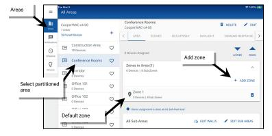
4: Type a descriptive name for the zone, and then select the zone type (dimmable, non-dimmable [switched], receptacle, or white tuning). **Zone type cannot be changed after initial setup**.
