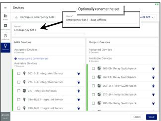
5: Assign up to 3 **NPS Devices** (Normal Power Sense) that will send the normal power signal beacons to the Emergency devices. Tap if to use **Blink to Identify** if needed to locate the correct device(s). Tap to place a **checkmark** next to the device(s) which will automatically move the device(s) to the Assigned Devices section.
