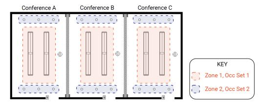
To create a new occupancy set in partitioned area and verify that they are properly assigned to the sub area(s):
