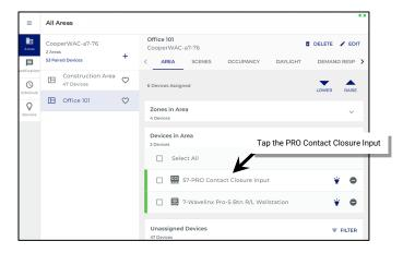
2: Verify that the device is set for the desired mode. If set for Contact Closure Mode, the screen will display four inputs. If set for Sensor Interface Mode, the screen will display occupancy sensor settings.
