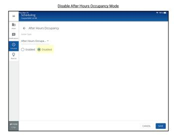
Only areas that are enabled for the After Hours Occupancy mode will respond with the unoccupied level change.
