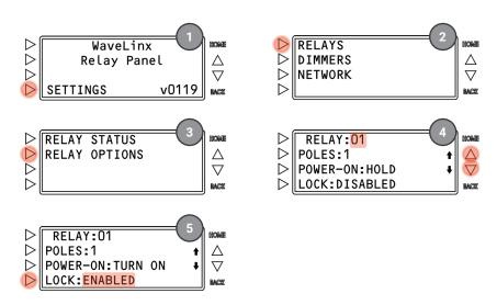
Once the lock is enabled through the onboard display, the physical relay lock switch can activate lock mode for the relay or return it to normal operating mode.
