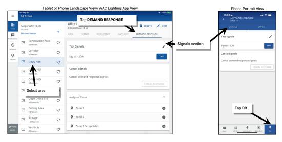
3: Tap edit / in the Test Signals section and then use the slider or number entry fields to enter the desired percentage of reduction. Tap SAVE.
