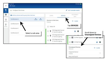
4: In the **Unassigned Devices** section, identify and then select the desired device(s). Tap • Add. For load control devices, when prompted select the sub zone.
