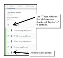
If multiple devices are selected, an additional bar will display at the bottom of the screen that shows the quantity of selected devices along with an option to identify or add the devices to the area. <sup>206</sup> **IMPORTANT! Verify that the quantity of devices selected is correct for the expected devices.** Tap • ADD to add the selected devices.
