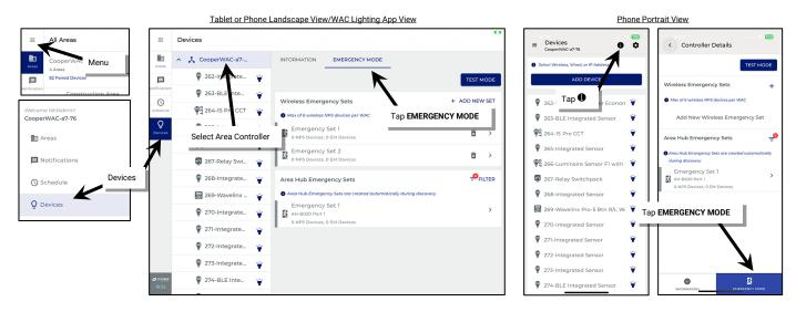
3: In the Wireless Emergency Sets section, locate the Emergency Set and then tap 🛍. When prompted, tap DELETE to confirm.
