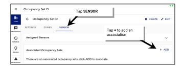
5: Locate the area(s) and tap > to expand the area(s) and show the occupancy sets. Select the occupancy set(s) that should pass commands to this one (for example, if zone D/occupancy set D needs to respond to commands from occupancy set A, select occupancy set A).
