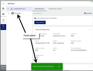
Repeat these steps to add additional Relay Panels to the WaveLinx Area Controller (maximum of 400 devices).
