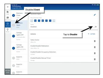
Re-enable the event by tapping the slider icon to switch the status to **Enabled**. The actions will execute the next time the event occurs.
