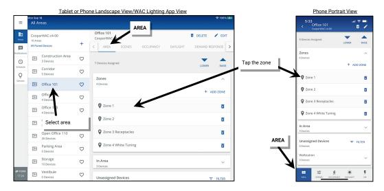
3: If there are multiple fixtures in the zone, identify the correct device using the device's identification method. For partitioned areas, the devices assigned sub area will be listed under the device name to help with identification. Refer to the device reference sheets starting on page 16 for details on the identification methods for that specific device. Once the device is identified, tap on the device to open it.
