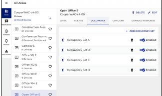
Associations are made between the occupancy sets controlling zone A, B, and C, to the walkway occupancy set D. (Remember, the general rule is to modify the occupancy set that needs to receive signals from other occupancy sets.) In this example, occupancy set D is associated with the other sets. During the association, the **Associated Occupancy Lighting Level** is set to **Enabled** and defined for a level of 20%.<sup>307</sup>
