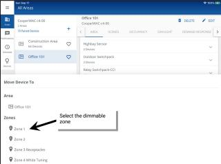
Use the drop down to select the appropriate zone for white tuning control (or for 2<sup>nd</sup> dimming zone for dual channel WaveLinx PRO Node). Verify that the zones are correct and then repeat for additional devices listed. Once all device channels are assigned, tap **SAVE**.
