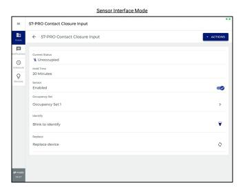
If the input type has changed, the device icon in the Devices In Area or Devices in Sub Area section may update to reflect the new input type.
