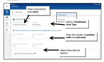
The number of walls and sub areas cannot be changed after the area is created. If the walls or sub areas are incorrect, delete the partitioned area and recreate it with the correct quantities of walls and sub areas.
