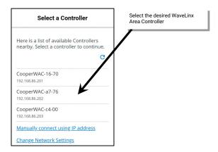
If no WaveLinx Area Controllers are found, touch the refresh button to begin the search again. If the touchscreen still does not find the WaveLinx Area Controller, select the option to **Manually Connect Using an IP Address**, and then type in the WaveLinx Area Controller's IP address. Tap the **SEARCH** button to connect to the WaveLinx Area Controller.
