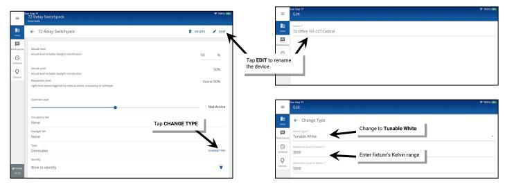
4: For both standard and partitioned areas, in the main area screen, tap on the previously configured white tuning zone. The white tuning Switchpack should now appear under **Devices in Area** or **Devices in Sub Area**. Tap on • to add the device to the white tuning zone.
