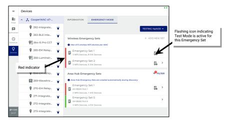
During the test, the Mobile App will display the active Emergency Test Mode in the Alerts Center.
