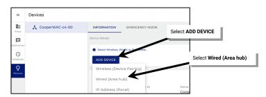
4: Wait for the search to complete and then review the Area Hub list; ensure that the desired area hub(s) is displayed by reviewing the area hub name, IP address, and/or MAC address. Tap the row for the desired **Area Hub**.
