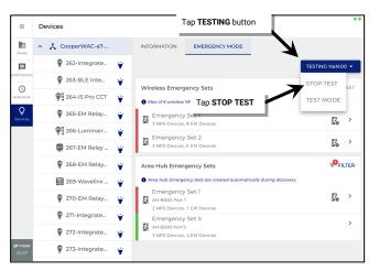
When the Emergency Set exits Test Mode, the EM devices will resume normal operation along with other normal power devices.
