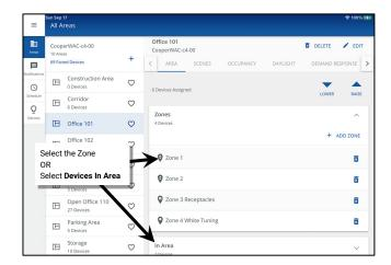
3: Select the desired device(s), and then tap • REMOVE. If removed from the Devices in Area section, the devices will automatically be moved to the Construction Area removing it from the user defined area. If removed from a zone, choose between moving the device into the Devices in Area section (ready to assign to another zone in the same area) or to the Construction Area removing it from the user defined area. Notifications will be displayed regarding the move.
