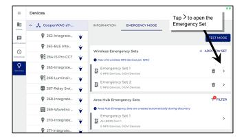
2: Assign/Unassign the **NPS Device(s)** (Normal Power Sense) that will send the normal power signal beacons to the Emergency devices. Tap to use **Blink to Identify** if needed to locate the correct device(s).
