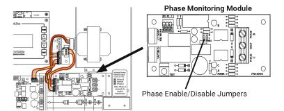
Panels ordered in an Emergency configuration will have special Relay Bypass Output Modules installed. This special output module allows selection of emergency operation of each relay output attached to that output module. The selection of operation is done using two rows of four jumpers. The jumpers ship in the default state to have all relays FORCE ON when the panel loses normal power. This allows any relays fed from emergency circuits to close allowing emergency loads to respond.
