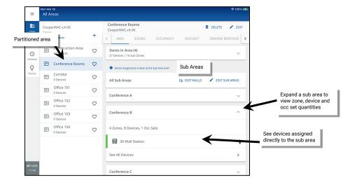
In the sub area section, tap on **PEDIT SUB AREAS** to view configuration screens for the sub areas. Change the name of the sub areas or in each sub area, view and change sub zone assignments, view or change device assignment, and view or change occupancy set assignments.
