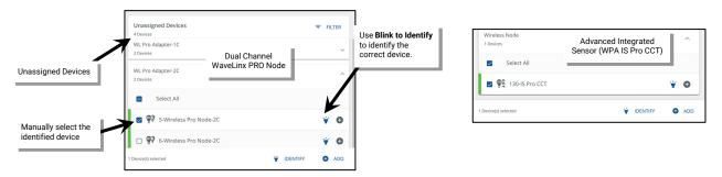
4: Verify that the device is the only device selected and then tap + or Add. (It is possible to add multiple devices at the same time using the multi-select feature. Please see "Using Multi-Select During Device Assignment" on page 172 for more information on using this feature).
