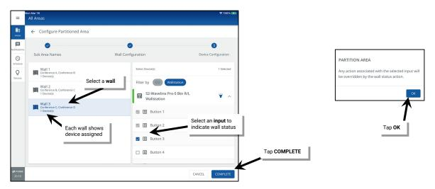
IMPORTANT: The device(s) that contains the inputs being assigned to the wall action WILL NOT be moved from their previously assigned area. If the devices are left in the construction area, there is risk of them being removed when devices are cleared from the construction area. To avoid this, make certain to assign the wall input device(s) to one of the partitioned sub areas.
