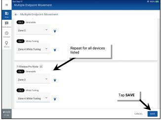
WaveLinx PRO Node devices only: If device configuration does not match default channel configuration (CH1 Dimmable, CH2 White Tuning) assign both channels to the area. Review steps in the previous section to reassign the channel type and then assign channels to the appropriate zones.
