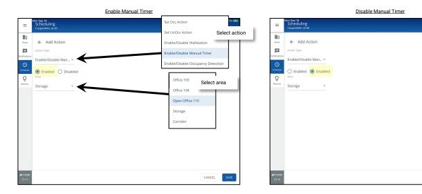
If a **Disable Manual Timer** event action is used, the timer and blink warns will not operate until an enable manual timer event action is processed. Remember to set an **Enable Manual Timer** event action at the time when the automatic timer shutoff should become operable. When the manual override timer is enabled and lighting is ON, the defined timer will restart so that lighting will automatically shut off once the timer expires.
