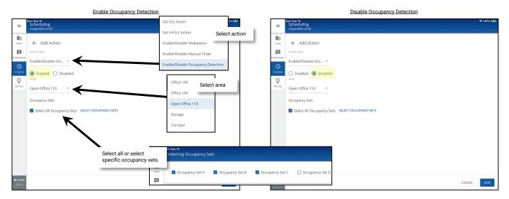
When a **Disable Occupancy Detection** event action occurs and the lighting is already ON due to the area being occupied previously, there will be no change in the current light level. If the lighting is in the unoccupied commanded level due to lack of motion and the **Disable Occupancy Detection** event occurs, the lighting will revert to the last commanded level prior to the unoccupied command. This is true regardless of whether the occupancy set is set to **Occupancy** or **Vacancy** mode.
