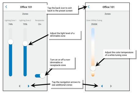
Note that partitioned areas will allow control from the Touchscreen with limited functionality. Commands from a Touchscreen to scenes and zones in a partitioned area will control lighting in the entire area regardless of partition wall open or close status.
