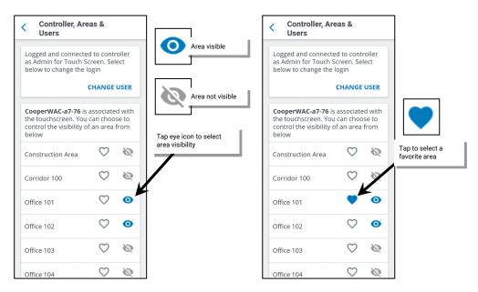
6: Tap the back button to exit and save the changes, and then tap the lock icon to exit the settings screen. The touchscreen should now show only the visible areas in the **All Areas** display.
