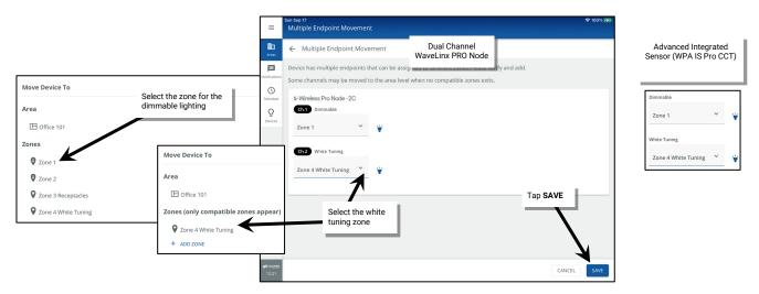
The WaveLinx PRO Node defaults to Channel 1 Dimmable, Channel 2 White Tuning (CCT range 3000-5000K). If the channel type <u>OR</u> default white tuning range (3000-5000K) is NOT correct see the next section "Changing Dual Channel WaveLinx PRO Node Configuration" on page 176.
