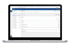
The WaveLinx Area Controller contains internal webpages that offer the ability to login via PC or device with a supported web browser to administer the lighting programming through the WAC Lighting App.
