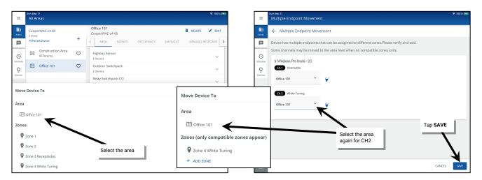
2. Locate and then select the device in the Devices in Area section of a standard area or the Devices in Sub Area of a partitioned area.
