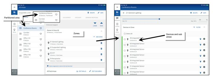
At the bottom of the main area screen are the area's sub areas. Expand any sub area to view the devices that are assigned directly to the sub area (typically wallstations, ceiling sensors and other input devices) and the quantity of sub zones, devices and occupancy sets that are assigned to that sub area.
