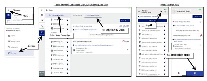
3: In the Wireless Emergency Sets section, tap ♣ ADD NEW SET or ♣. The new set will be added to the Wireless Emergency Set list.
