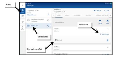
3: Type a descriptive name for the zone, and then select the zone type (dimmable, non-dimmable [switched], receptacle, or white tuning). **Zone type cannot be changed after initial setup**.
