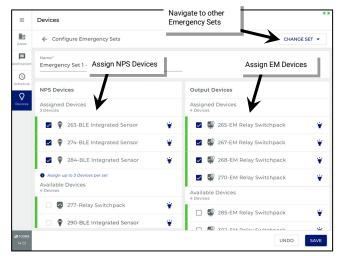
The WaveLinx Wireless Emergency Sets and Area Hub Emergency Sets have a colored indicator bar at the beginning of the Emergency Set Row. The colored indicator bar can be gray, red, or green. These colors can indicate different conditions:
