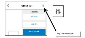
It is also possible to adjust individual zone light levels or white tuning color temperature. To access the zone adjustments, tap the zone level icon at the top of the area presets screen.
