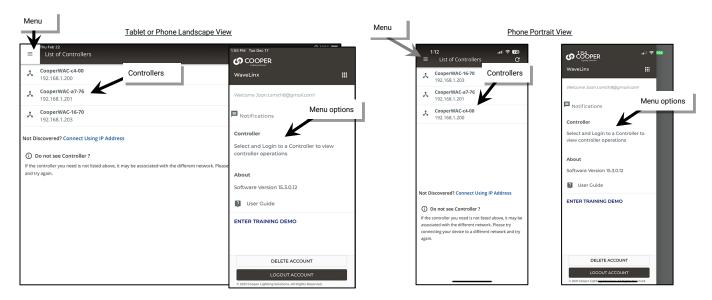
The **List of Controllers** is used to open a WaveLinx Area Controller for programming. Multiple WaveLinx Area Controllers may appear if the site has multiple connected to same network that the mobile device is accessing.
