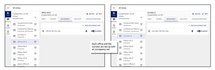
Associated Occupancy Lighting Level settings are available when using WaveLinx Area Controller firmware version 10.0.x.x and higher. Previous version WAC's will not show the Associated Occupancy Lighting Level option. If an association is made and an associated occupancy set issues a command, the lighting will respond with the programmed occupied action.
