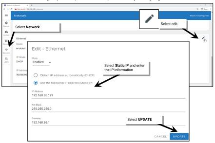
The WaveLinx Area Controller initial setup is complete.
