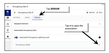
5: Locate the area(s) with the associated occupancy set(s). Tap > to expand the area(s). Uncheck the occupancy set(s) that no longer needs to be associated and then tap **SAVE**.
