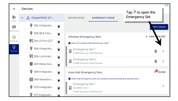
2: Assign or Unassign the **Output Devices** (Emergency Devices) that will respond to the NPS devices in this set. Tap \*\* to use **Blink to Identify** if needed to locate the correct device(s).
