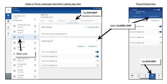
3: Tap the option to CALIBRATE ALL. All enabled closed loop daylight set lighting devices will go to their brightest light output.
