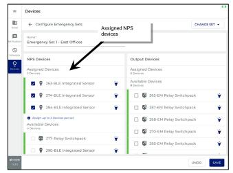
6: Next, assign the **Output Devices** (Emergency Devices) that will respond to the NPS devices in this set. Tap \* to use **Blink to Identify** if needed to locate the correct device(s). Tap to place a **checkmark** next to the device(s) to move them to the Assigned Devices section.
