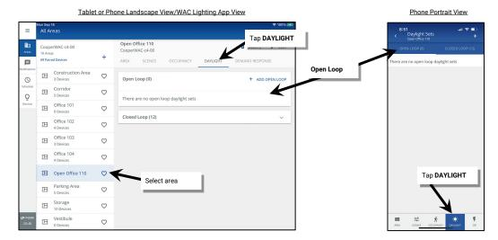
3: Tap + to add an open loop daylight set, and then tap the new daylight set to open it.
