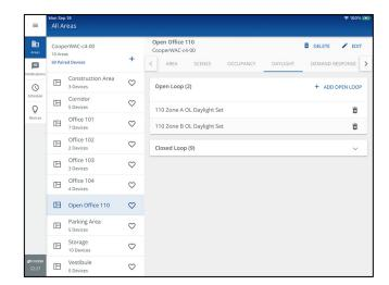
Two open loop daylight sets are programmed in the area.
