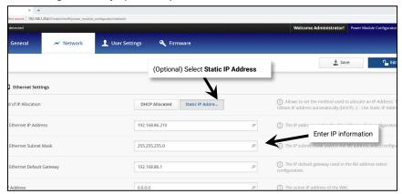
6: In the appropriate tab (either DHCP or Static IP depending on which the site is using) enter the IP address of the WaveLinx Area Controller that should be paired with this Low-Voltage Power Module in the WAC IP Address field. This ensures that the Low-Voltage Power Module will pair with the correct WaveLinx Area Controller.
