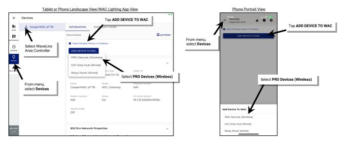
During the 60-minute pairing period, WaveLinx PRO devices and the WaveLinx Low-Voltage Power Module should pair with the WaveLinx Area Controller. Devices should exhibit the successful paired device behavior described in the device reference sheets.
