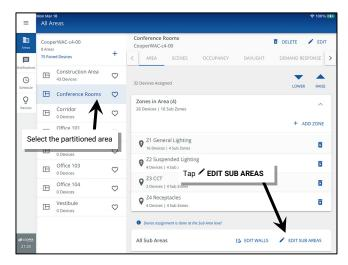
3: Select the **sub area** and tap on **DEVICES** to view the **Devices in Sub Area**. Identify and select the desired device(s) and tap **Remove.** The device(s) will be moved to the Construction Area.
