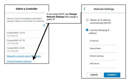
5: Once it has an IP address, the touchscreen will search for and then display any WaveLinx Area Controllers that it has found on the network. If the site has more than one WaveLinx Area Controller, multiple WaveLinx Area Controllers may be listed. Select the WaveLinx Area Controller that is programmed for the area(s) that the touchscreen should operate.
