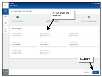
5: Perform the **Wall Configuration**. Tap any **Wall Name** to change the default name and then use the drop down to **select the sub areas** that the wall joins (must select at min. two sub areas, max. ten sub areas). Repeat until all wall names and sub areas are defined. Tap **NEXT** to move on to the next step.
