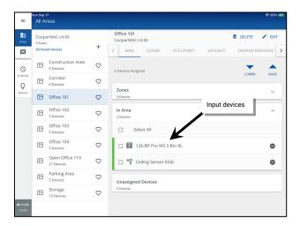
If devices have not been assigned to an area, they will appear in the Unassigned Devices section or in the Construction Area.
