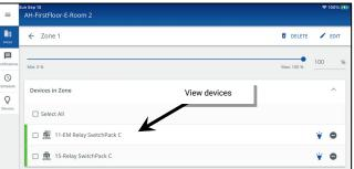
5: Tap Devices in Area to show additional devices such as wallstations, ceiling sensors, and interface modules. Tap a device to view it.
