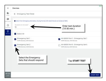
When the test is started, all EM Devices from the selected Emergency Sets will turn ON/100% and will not respond to other WaveLinx Device commands. WaveLinx wallstations can be used to verify proper response. If wallstations are used, the normal lighting will respond but the EM devices will remain ON/100%.
