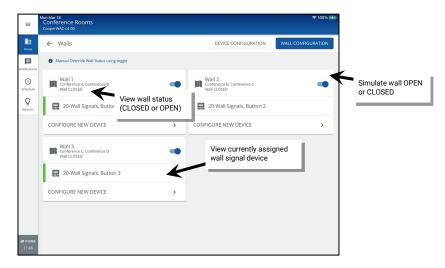
Tap **DEVICE CONFIGURATION** to change the device currently mapped to each wall.
