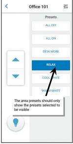
The touchscreen can now be used to control lighting in the defined areas. For information on the screen controls, refer to "Using the Touchscreen Controls" on page 328.
