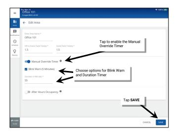
Only zones that are not assigned to occupancy sets will respond to the manual override timer. Make sure to remove zones that should respond to the manual override timer from the occupancy set assignment.
