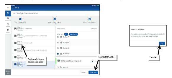
IMPORTANT: The device(s) that contains the inputs being assigned to the wall action WILL NOT be moved from their previously assigned area. If the devices are left in the construction area, there is risk of them being removed when devices are cleared from the construction area. To avoid this, make certain to assign the wall input device(s) to one of the partitioned sub areas. See page 173 for instructions.
