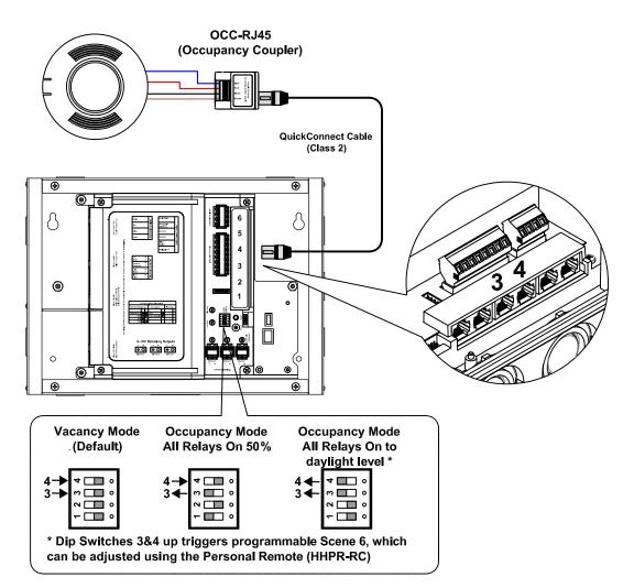
Control Sequence: Code requires that lighiting be either turned ON Manually or can be Automatic ON. Title 24 provides additiona PAF credits if the lighting is turned on to no more than 50%. The Room Controller supports all of these functions. Out of the box the Room Controller arrives in Vacancy Mode.
