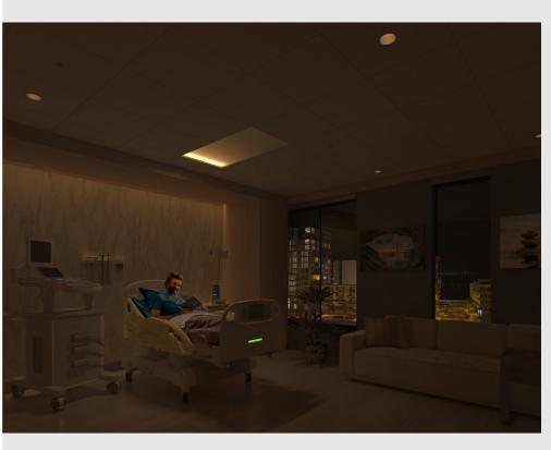
Nightlight should reflect the sunset lighting spectrum, with primarily light colors in the red, at a low intensity. Once people are sleeping, the light shouldn't be higher than 1 lux, which is equivalent to the light of a candle.
