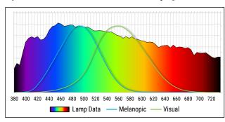
With melanopic lighting, the melanopic DER is 42% higher compared to the standard LED spectrum. There's no change in visual color impression or visual light output between melanopic and LED lighting. This graph shows the peak in the cyan wavelength, aligned with biological active light.
