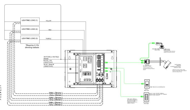
\*0-10V Dimming Zone Note: The 0-10V dimming zones within the Room Controller can be wired and controlled independent of the connected loads. This allows a each load to have a dedicated 0-10V dimming zone or a single load to have up to three 0-10V dimming zones.
