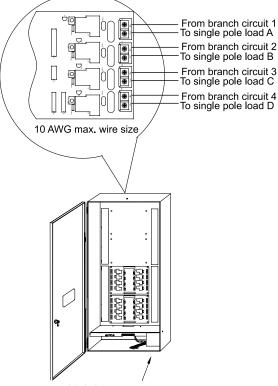
Lighting control panel power supply: 120/277 VAC double tap transformer standard 120/347 VAC double tap transformer is available for Canada
