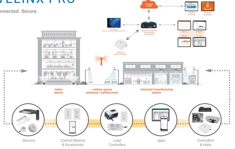
WaveLinx PRO is a distributed wireless lighting control system that eliminates the need to run control wires to each device, lowering installation costs by up to 40%.
