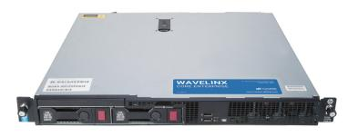
WaveLinx CORE Enterprise / WaveLinx Virtual CORE Enterprise The WaveLinx CORE Enterprise is an on-premise hardware platform hosting CORE software applications. They network up to three-hundred (300) WaveLinx Area Controllers or 32,500 devices, collecting data that can be shared with third party system via BACnet and Public API (REST).
