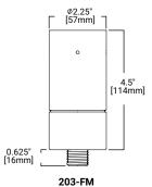
TECHNICAL DATA 8W LED, L70/60,000 hours at 25°C Low Voltage: 50W Halogen MR16
