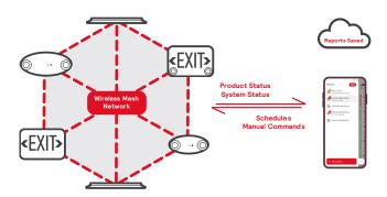
FirstLink is a standalone wireless system which integrates all necessary emergency lighting components with an app installed on a tablet or smartphone.
