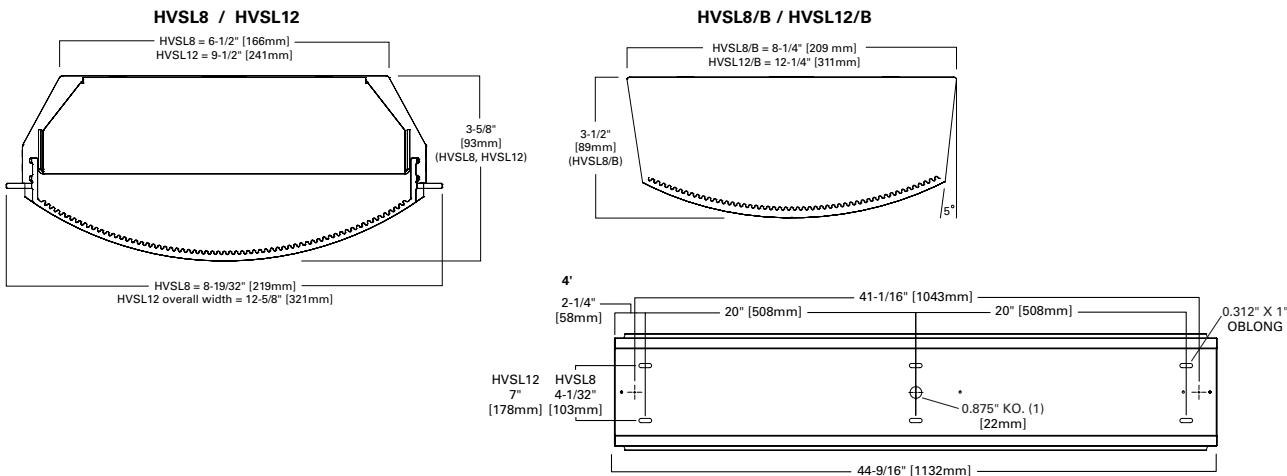
(8' unit consists of (2) 4' units, attached at the factory)
