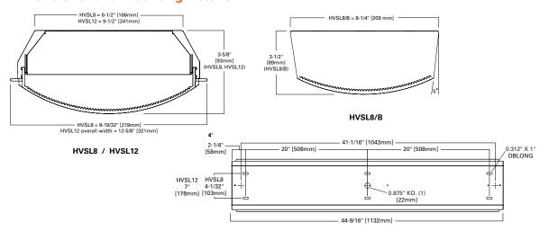
(8' unit cnsists of (2) 4' units, attached at the factory)
