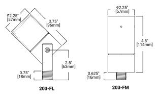
**TECHNICAL DATA** 8W LED, L70/60,000 hours at 25°C Low Voltage: 50W Halogen MR16
