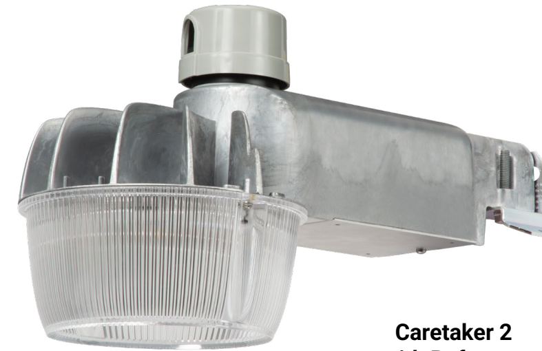
Caretaker 2 with Zero Uplight Shield Max Lumens @ 4000K: 12,200 HID Replacement: up to 150W Weight: 7 lbs
